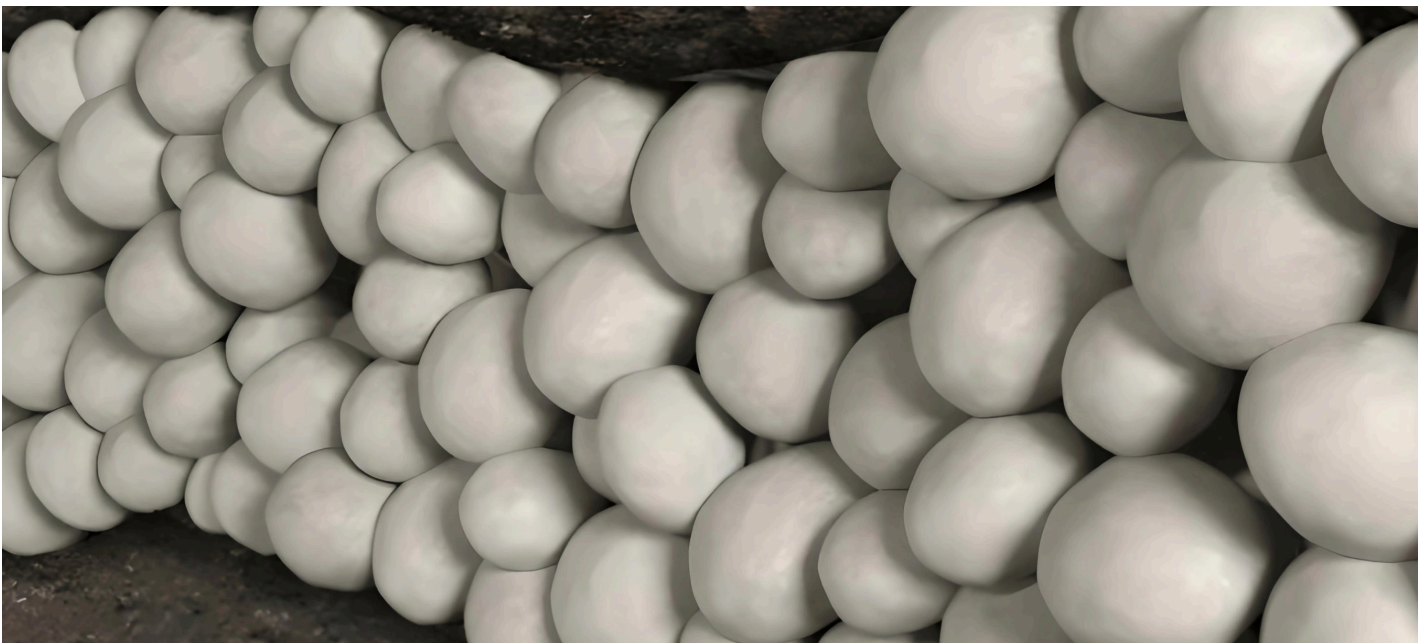
In an enhanced geothermal system, propped fractures form an artificial heat exchanger that must stay open and conductive for decades.
